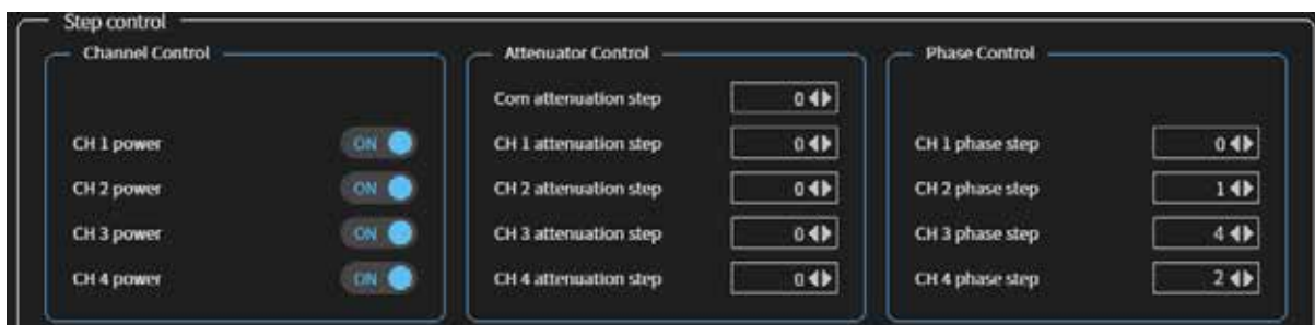
Figure 14. Phase Control for Boresight
