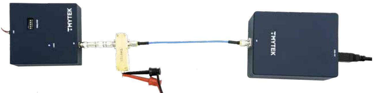
Figure 8. PLO + Attenuator + Adapter + Amplifier + Cable
