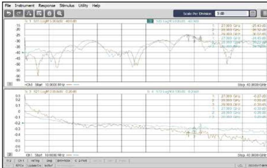
Figure 9. S-Parameter of the Adapter
