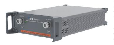
BN100 USB Vector Network Analyzer offers wide dynamic range, low noise level, high resolution scanning with laboratory and research grade performance. BN100 covers frequency range from 1MHz to 6.5GHz with 2-port and 2-path that competitive with most of the bench-top VNAs on the market. BN100 USB VNA provides measurement convenience by offering end user excellent performance and attractive price. BN100 VNA is suitable for laboratory, manufacturing and many other safety testing environment.
